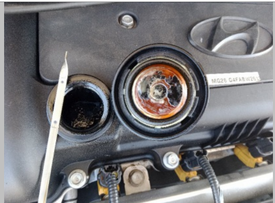
Oil filler cap and dipstick
